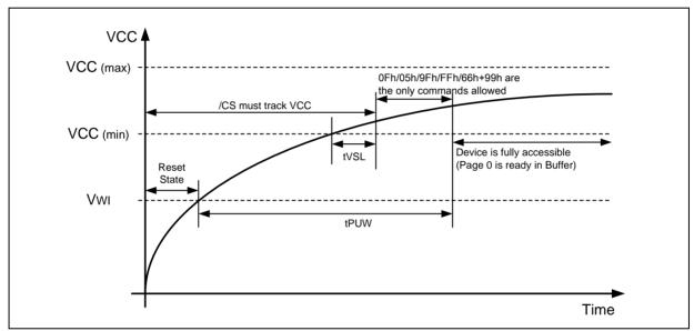
Figure 33a. Power-up Timing and Voltage Levels
