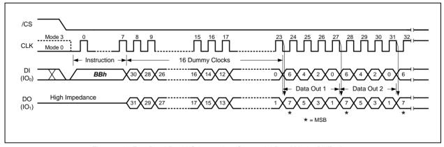
Figure 26b. Fast Read Dual I/O Instruction (Sequential Read Mode, BUF=0)
