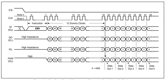
Figure 28b. Fast Read Quad I/O Instruction (Sequential Read Mode, BUF=0)
