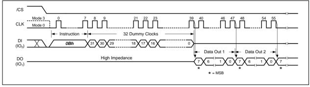
Figure 20b. Fast Read Instruction (Sequential Read Mode, BUF=0)
