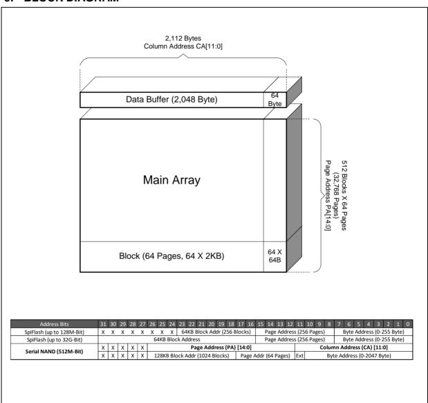
Figure 2. W25N512GW Flash Memory Architecture and Addressing
