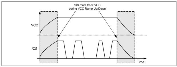
Figure 33b. Power-up, Power-Down Requirement
