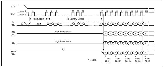
Figure 25b. Fast Read Quad Output with 4-Byte Address Instruction (Sequential Read Mode, BUF=0)
