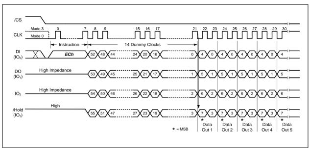
Figure 29b. Fast Read Quad I/O with 4-Byte Address Instruction (Sequential Read Mode, BUF=0)
