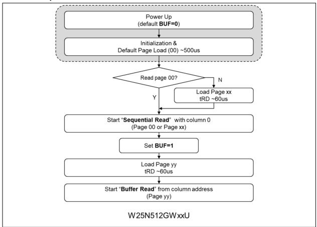
Figure 3. W25N512GW Flash Memory Operation Diagram
