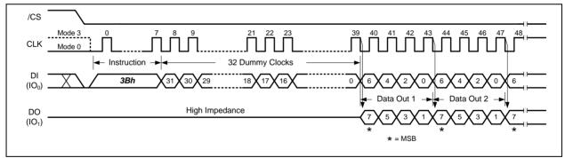
Figure 22b. Fast Read Dual Output Instruction (Sequential Read Mode, BUF=0)
