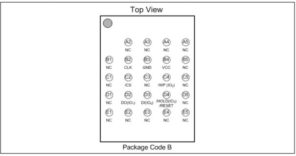
Figure 1b. W25N512GW Ball Assignments, 24-ball TFBGA 8x6-mm (Package Code B)
