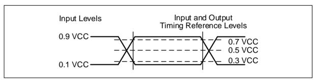
Figure 35. AC Measurement I/O Waveform
