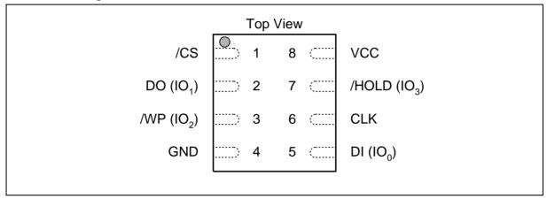
Figure 1a. W25N512GW Pad Assignments, 8-pad WSON 6x5-mm / 8x6-mm (Package Code P, E)
