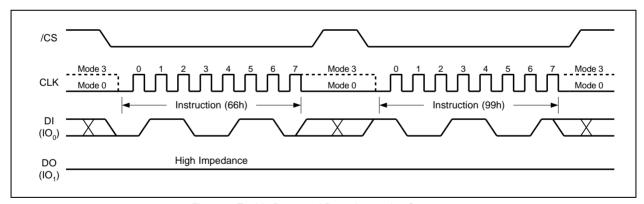
Figure 6. Enable Reset and Reset Instruction Sequence
