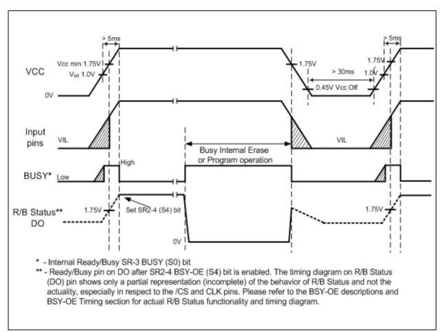
Figure 34. Power loss Timing and Voltage Levels
