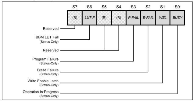
Figure 4c. Status Register-3 (Address Cxh)
