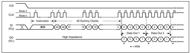
Figure 23b. Fast Read Dual Output with 4-Byte Address Instruction (Sequential Read Mode, BUF=0)
