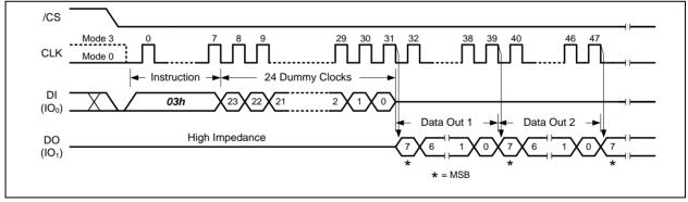
Figure 19b. Read Data Instruction (Sequential Read Mode, BUF=0)
