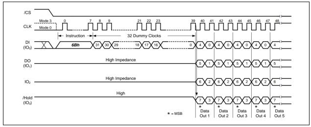
Figure 24b. Fast Read Quad Output Instruction (Sequential Read Mode, BUF=0)
