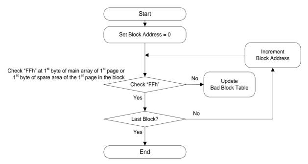
Figure 36. Flow chart of create initial invalid block table
