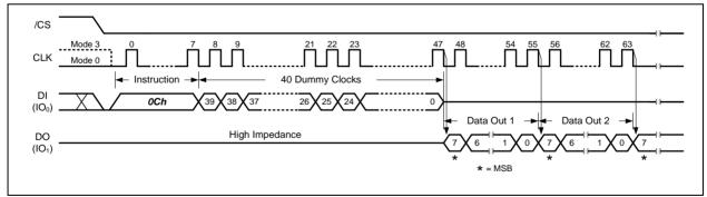
Figure 21b. Fast Read with 4-Byte Address Instruction (Sequential Read Mode, BUF=0)
