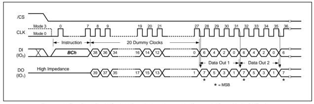
Figure 27b. Fast Read Dual I/O with 4-Byte Address Instruction (Sequential Read Mode, BUF=0)
